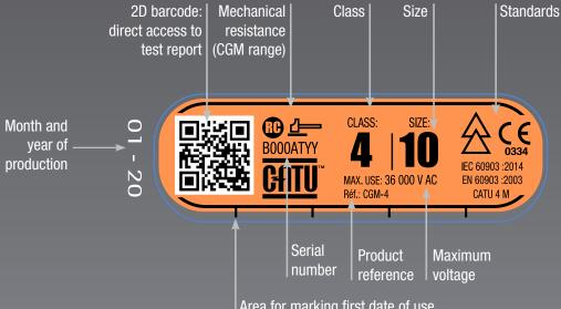
Area for marking first date of use and subsequent test dates
